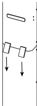
3 Carefully insert the camera tower into the base
