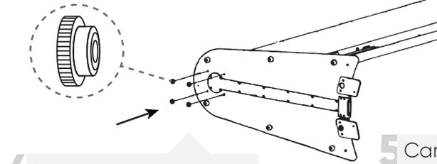
4 Attach 4 thumb nuts to secure camera tower
