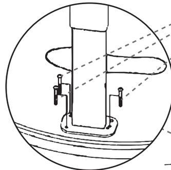
4 Use Allen key (included) to tighten screws
