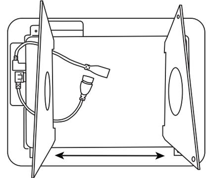
4 Route the cables underneath the mounting bracket as shown
