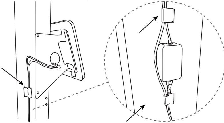
8 Connect the USB cable to the camera tower
