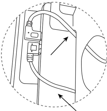
5 Connect the tablet power supply and the USB cable to the adapters. Route the cables through the round hole of the mounting bracket on the right as shown
