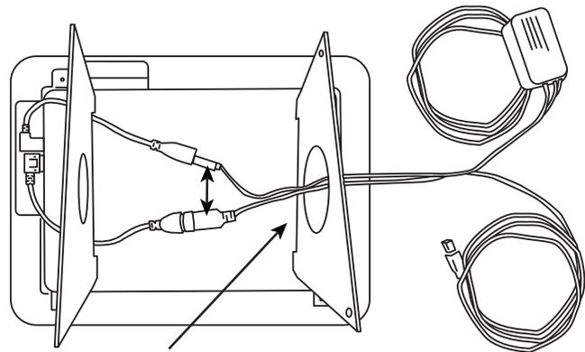
6 Remove the four small screws from the camera tower located along the rear edge above the center camera location. Use four of the longer screws included with the tablet accessories to attach the tablet assembly to the camera tower
