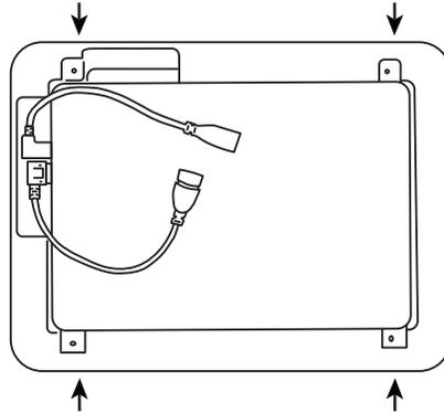
3 Attach the left and right mounting brackets to the bezel with four of the included screws
